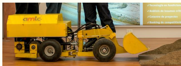
Figure 12. 1:5 scaled LHD built for testing and validation.
